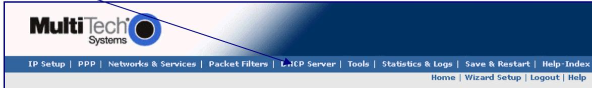
**IP Setup:** Sets up a General Configuration, HTTP, DDNS, SNTP, Static Routes, and Remote Configuration.
